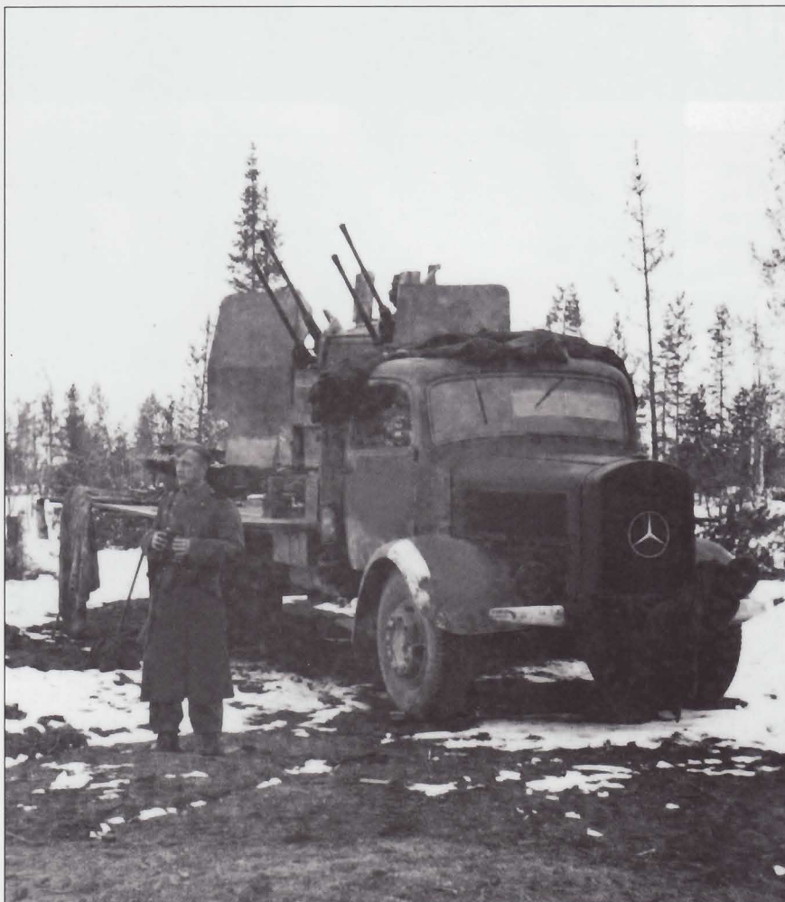
Two photographs of a 2cm FlaK38 Flakvierling mounted on a Mercedes-Benz L3000 truck. Note the registration plate and white road markings that were used until 1943. This particular flak gun was normally served by an eight-man crew. These quadruple weapons were much respected by low-level enemy pilots and were devastating against light vehicles, as well as troops caught in the open. (MK photo)
