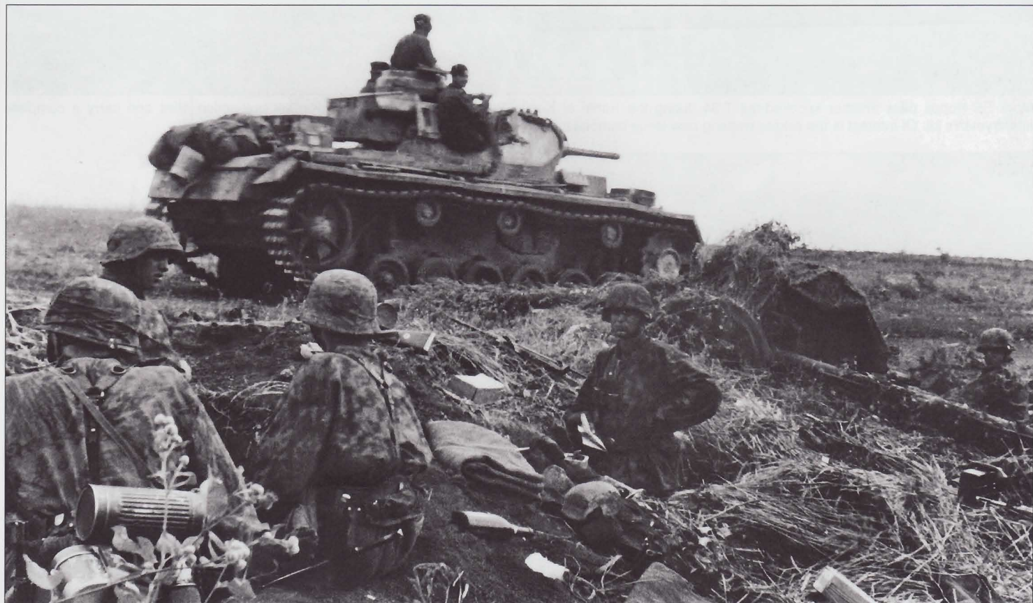
A gun crew with their heavily camouflaged 7.5cm PaK40 gun is dug in during bitter fighting against strong Soviet positions. A Pz.Kpfw.III Ausf.J armed with a 5cm L/42 gun passes a group of antitank gunners wearing the "oak leaf" and "palm tree" pattern camouflage smocks. One soldier on the left, however, is wearing an early-style "palm" pattern camouflage smock.
