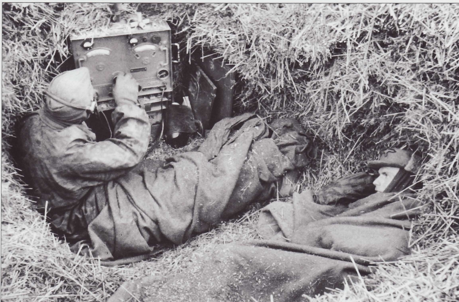
In a well-concealed dugout, Waffen-SS radiomen can be seen with their Torn. Fu. B1 S/E radio in the winter of 1943. These widely used portable radios were carried by a soldier on a specially designed backpack frame, and when connected to each other (upper and lower valves) via special cables, they could be used on the march.
