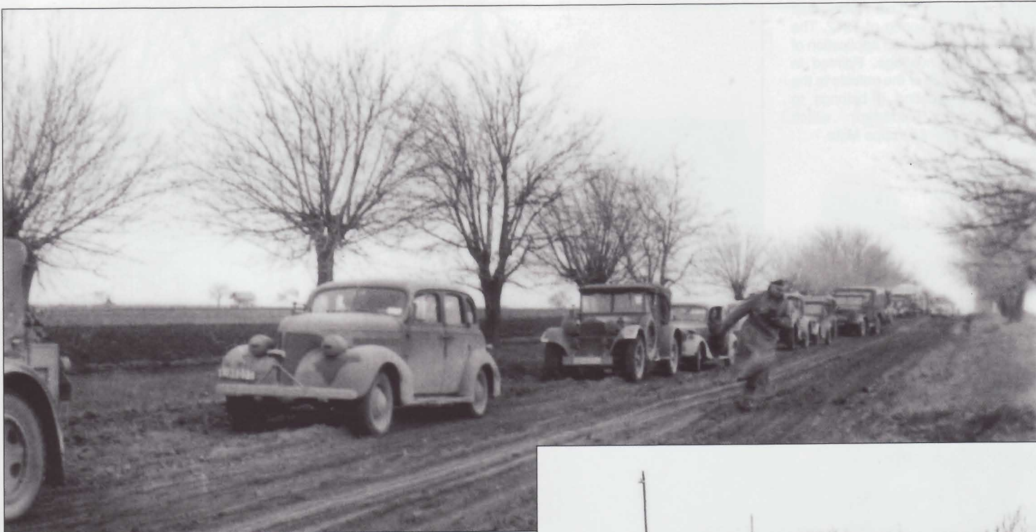
A long column of SS staff cars in Heeresgruppe Mitte struggling along a muddy road in Russia during the early spring of 1942. Note the second car from the left. This is a Chevrolet limousine that has been pressed into service by the German Army. It has been repainted in dark gray and is covered with mud. The car is equipped with an improvised Notek light installed on a guard in front of the radiator. Behind the Chevrolet, a standard medium personnel carrier follows.
