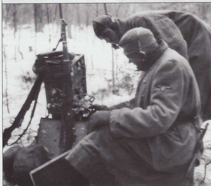
"Das Reich" radiomen in a forest with a Tornisterfunkgerät b1 (Torn. Fu. b1 (S/E), or "pack radio". These portable radio sets were widely used on the Eastern Front and were carried by radiomen in two parts on specially designed backpack frames.
