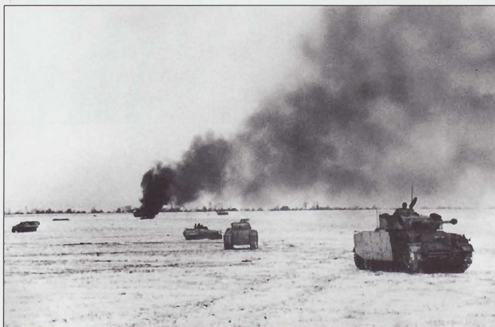
German armored vehicles of the SS-Kampfgruppe in a snow-covered field following heavy action against an enemy target. All the armored vehicles have received an application of winter whitewash paint. The Pz.Kpfw.IV in the foreground has obviously been embroiled in some heavy enemy contact and has lost part of its Schürzen as a result.
